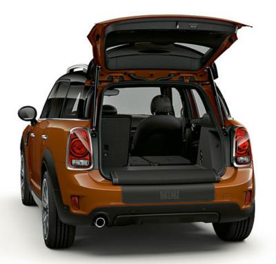
You can use the luggage space in the MINI Countryman in any number of ways: the load-compartment floor folds away and the rear backrests fold down in a 40:20:40 split. The rear seat bench slides forward to provide even more room, and splits in a 40:60 arrangement.
