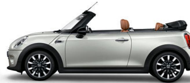
The soft top of the MINI Cabrio opens electrically in 20 seconds – even with the car moving at up to 30 km/h. When the top is closed the multiple layers of fabric make for excellent sound insulation and comfort on long journeys.
