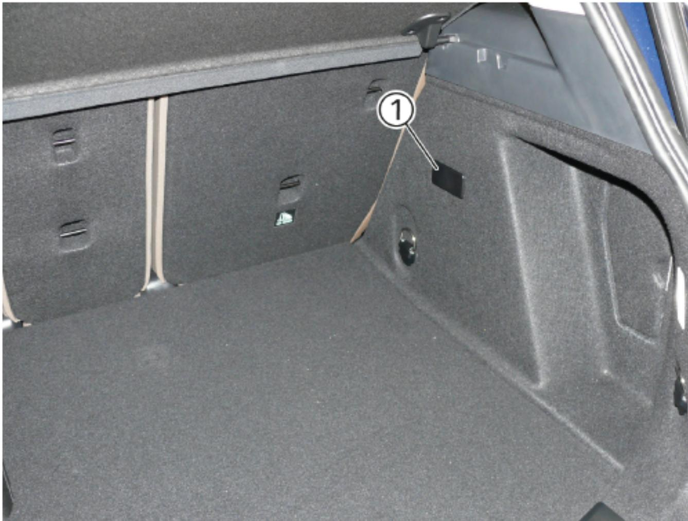
Press the connector switch fuse (1) downwards and pull it out. Disconnect the connector for the high voltage disconnect (2) (Service Disconnect) in the direction of the arrow.
