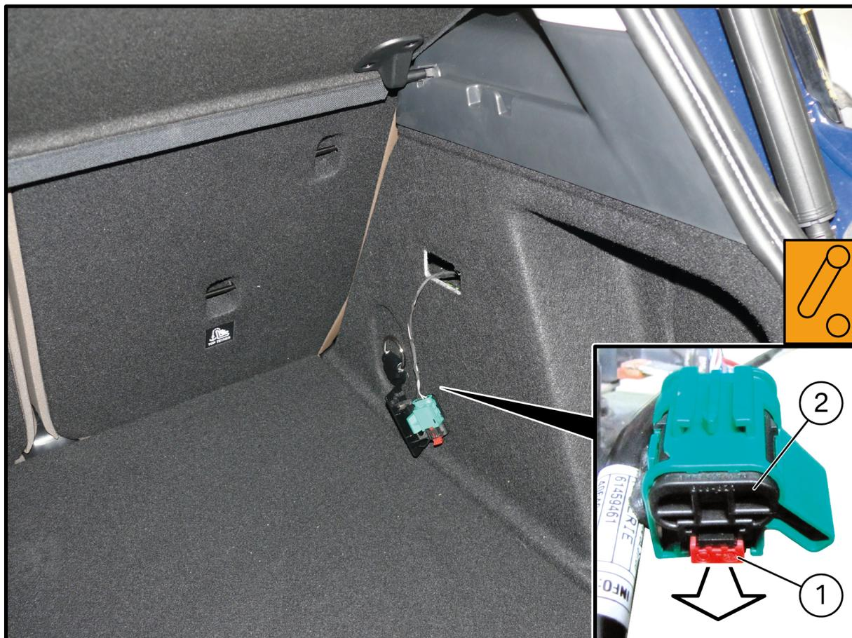
The high-voltage system is deactivated when bore hole (1) is completely free.
